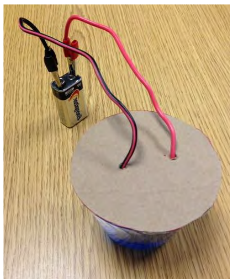
Figure 9. A) Cross section illustration of final copper electrolysis lab set-up. B) Actual copper electrolysis lab set-up.
