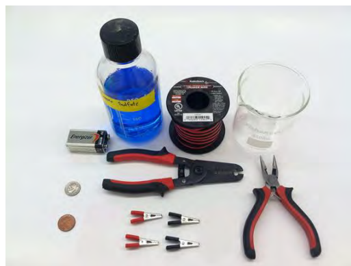
Figure 1. Materials needed for copper electrolysis lab.
