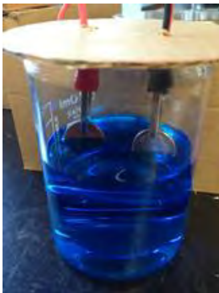
Figure 8. Electrodes immersed in the electrolyte solution
