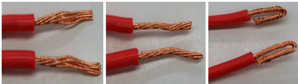
Figure 5. A) Exposed copper filaments; B) twisted copper filaments; and C) final product of twisted and folded copper filaments.
