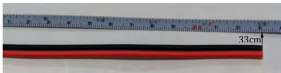
Figure 2. 33 cm length of 18-gauge copper wire.
